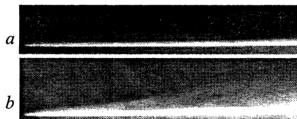
Fig. 7. Side view of a surface microwave discharge on the top part of the flat antenna streamlined by a supersonic stream of air (a) and propane-butane-air mixtures (b) at M = 2 , p = 40 torr, \tau = 100 \mu s and pulsed microwave power W_p = 40 kW (mean power W_m = 40 W).
