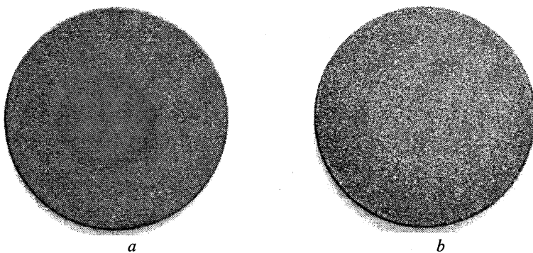
Fig. 4. Photographs of the diamond disks with silicon substrates grown in CW (a) and pulsed (b) regimes, deposition time is 100 h in both cases.
