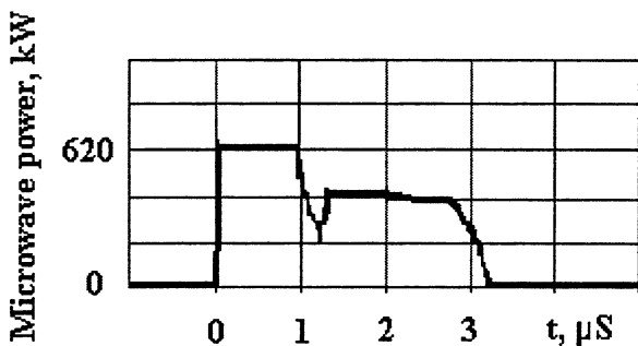
Fig. 3a. Oscillogram of the envelope of pulsed microwave power reflected from the discharge plasma.
